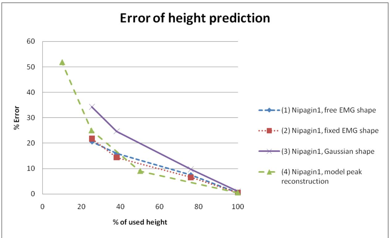
Figure 5. Peak reconstruction for Nipagin Series 1. For the fixed EMG shape  $\sigma$  and  $\tau$  parameters of the EMG were fixed to the values, obtained for the Model peak; free EMG shape allow  $\sigma$  and  $\tau$  to be optimized. The Model peak is the highest “normal” peak (peak with concentration of 4 in Series 1). “True” height and area were determined by the extrapolation of the calibration dependence.
