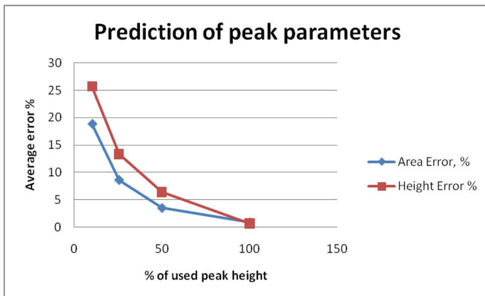
Figure 2. Prediction of the peak height and area for 44 stand-alone peaks from different chromatograms (all LC)
