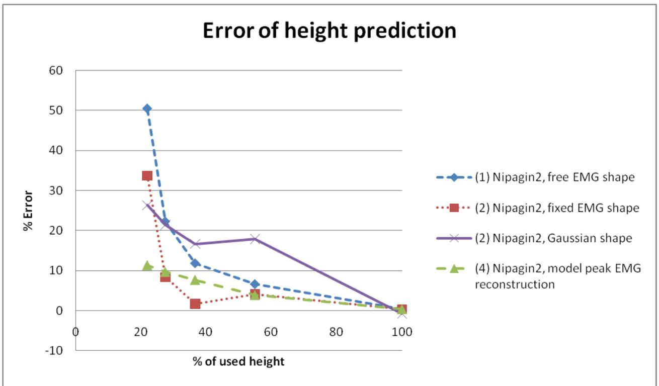
Figure 6. Peak reconstruction for Nipagin Series 2. Concentrations 1: 2: 3: 4: 5. Already, the second peak is out of the range. The “true” peak height was calculated by scaling of the Model (concentration = 1) peak height.
